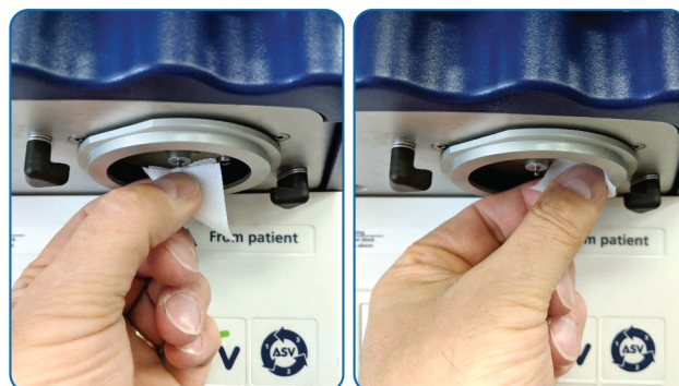
Figure 5. Cleaning the valve plunger and centering ring
